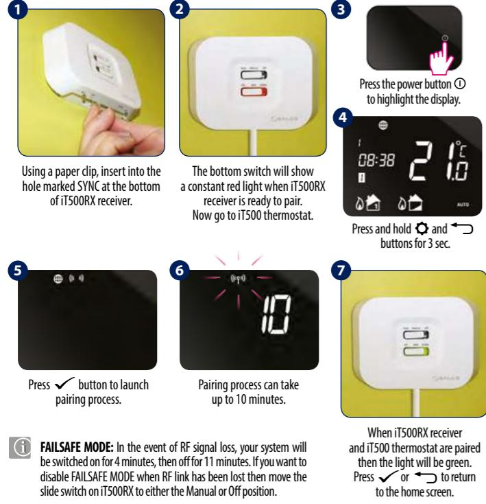
Using a paper clip, insert into the hole marked SYNC at the bottom of iT500RX receiver.
